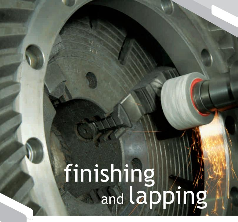
Gears are finished on most modern grinding machines and lapping is done with special lapping compound on PLC controlled most modern Gleason lapping with SPC (Swing Pinion Cone) action to improve surface finish resulting in noise free gears.
