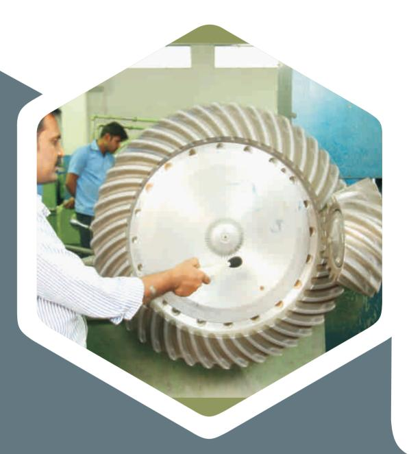
Finished goods are inspected as per specifications provided by Customer / International Standards. Highest level of quality is possible by imposing stringent measures starting from receipt of forgings to packaging stage. Tooth spacing, contact pattern noise level and backlash checks are performed using Gleason Testers and other related equipment. Finally it is the obsession with quality that has earned PLACEBO the privilege to supply gears to the OEM and various clients.
